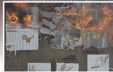
Figure 1 Fire spreading between dwellings
